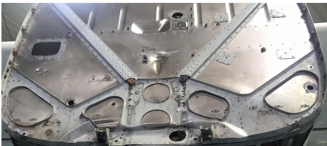
Figure 2. Firewall penetrations, openings and access panels.
