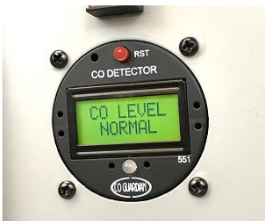
Figure 5. TSO approved panel mounted CO detectors.
